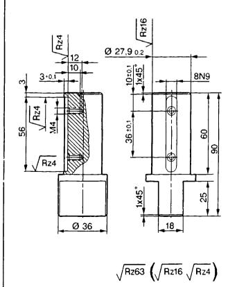
Clamping pin for drive spindle with multi-plate clutch
